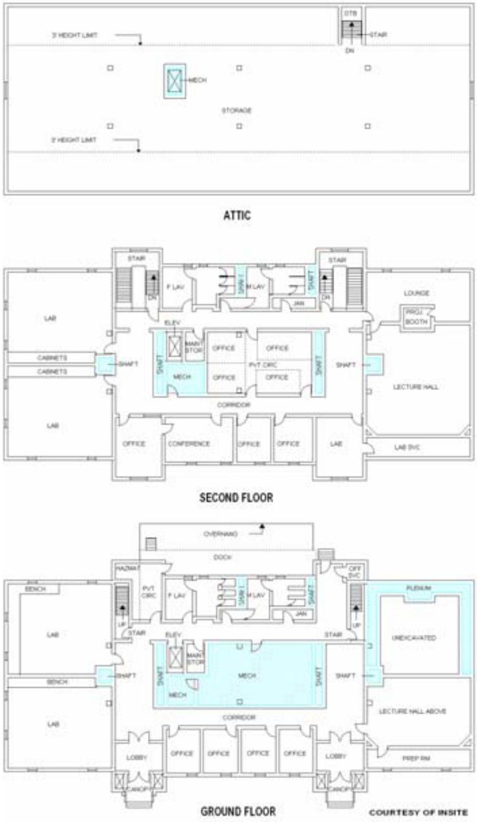
Figure 3-6. Mechanical Area of a building by floor
